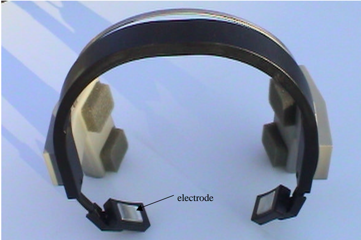
Figure 1. Headset with electrodes for transdermal electrical stimulation for tinnitus treatment is depicted. High frequencies were modulated on an ultrasonic carrier with the device (Theraband) capacitive coupled to the head during stimulation.
